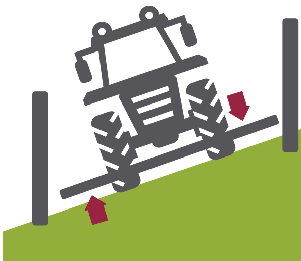
Figure 2-1: Double-sided weeding is impractical on rows that run across a hill slope. The two sides of the implement will hit the ground at different heights.
