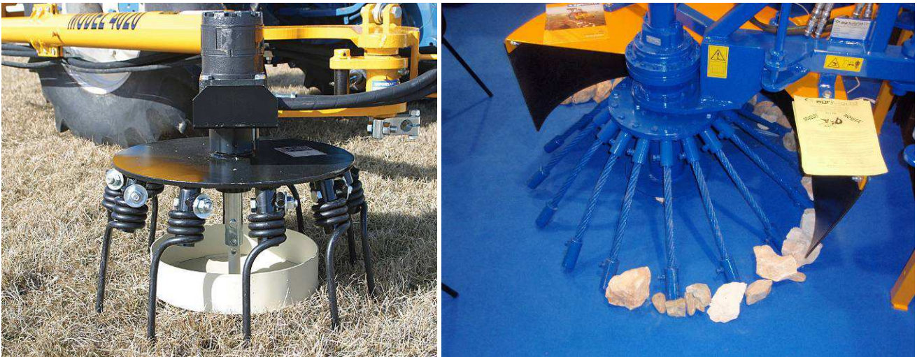
Figure 5. Powered undervine cultivators: left, vertical spring rods, right, vertical axis wire brush.
