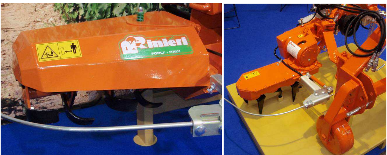
Figure 4. Powered undervine cultivators: left, rotary hoe / rotovator type, right, vertical power harrow type.
