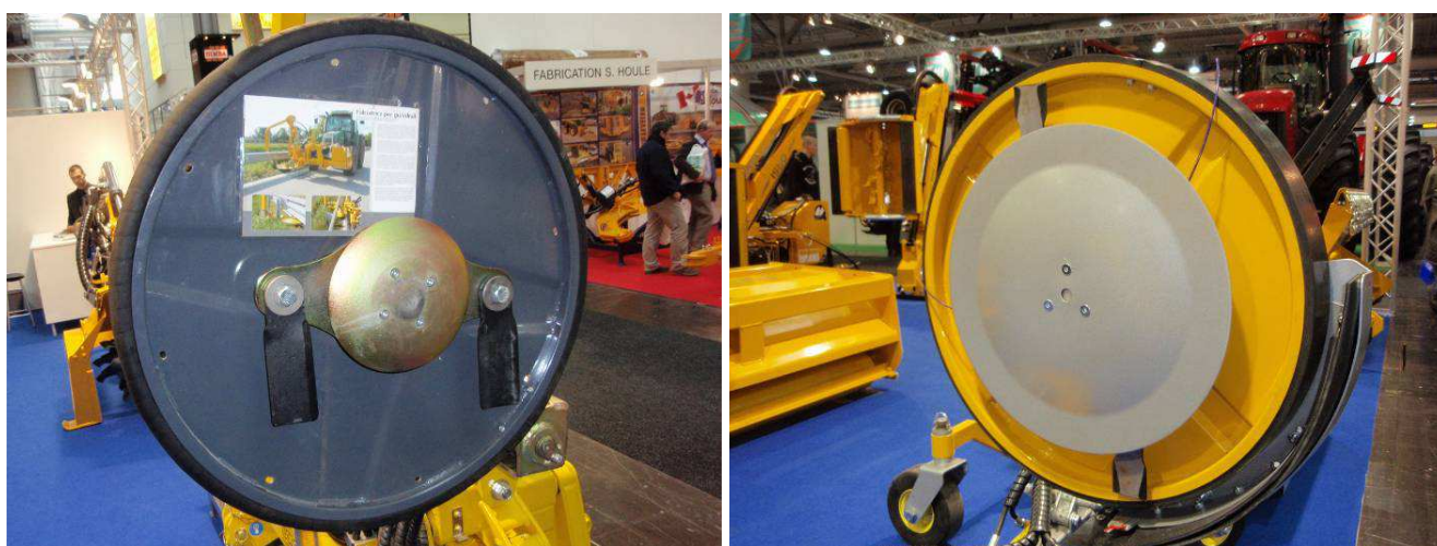
Figure 2. Examples of vertical axis, horizontal blade system in undervine mowers.
