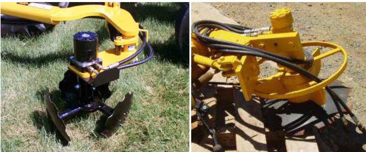
Figure 6. Powered undervine cultivators: left, vertical axis vertical rotating disks ('cyclone'), right, vertical axis horizontal rotating disk.
