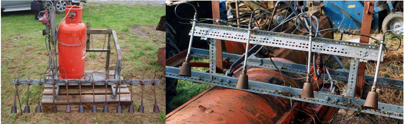
Figure 5. Simple un-hooded tractor mounted flame weeder comprised of multiple torch heads to treat the whole bed (left) or to just treat the crop rows (right).
