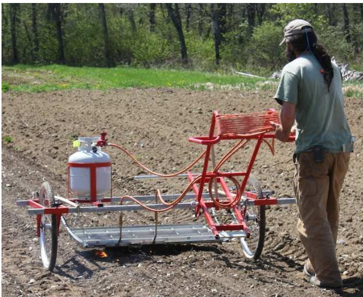
Figure 4. Pedestrian propelled bed flame weeder (photo courtesy of Dr Eric Gallandt).
