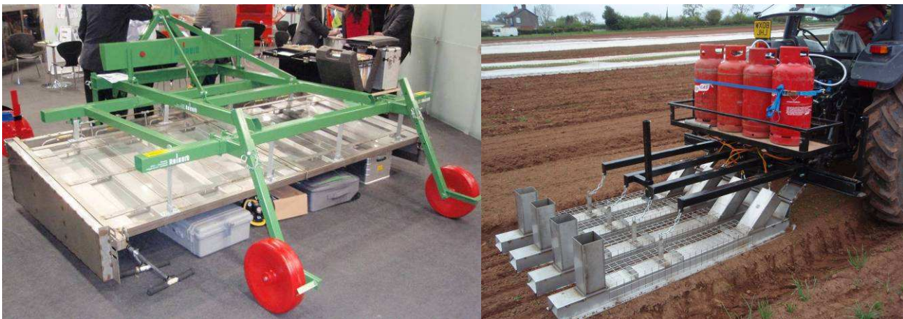
Figure 7. Hooded whole-bed flame weeder design (left), intrarow design (right).
