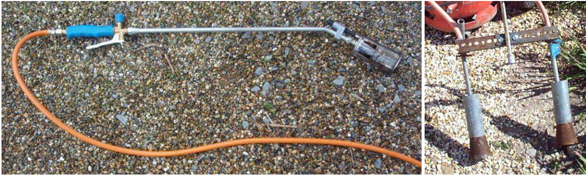
Figure 3. Typical hand-held builders torch (left) twin burner setup (right).
