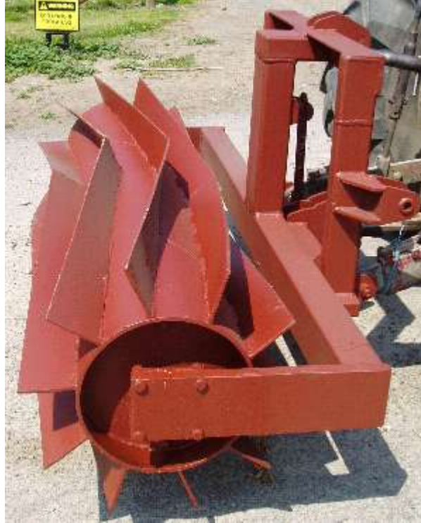
Figure 1. North American helical crimper roller design as built for this trial.
