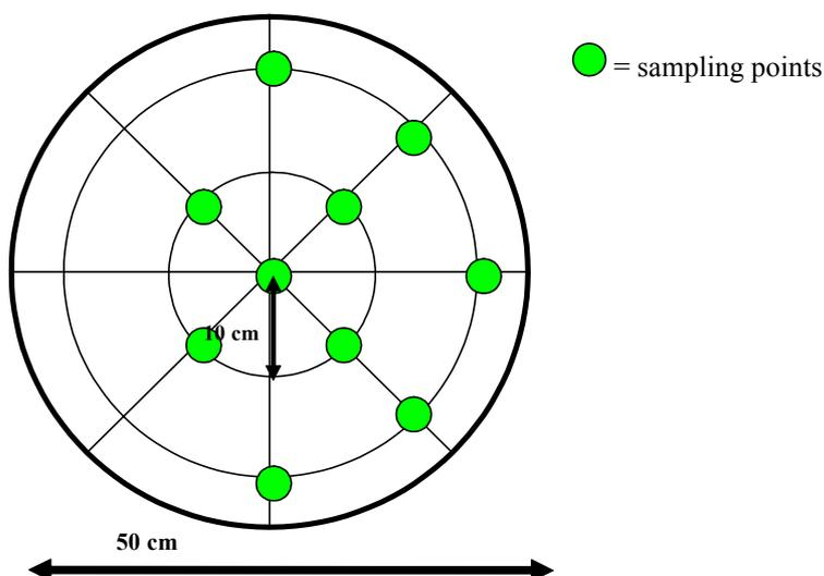
**Figure 10: Sampling design tested to determine spatial variability pattern in lysimeters.**
